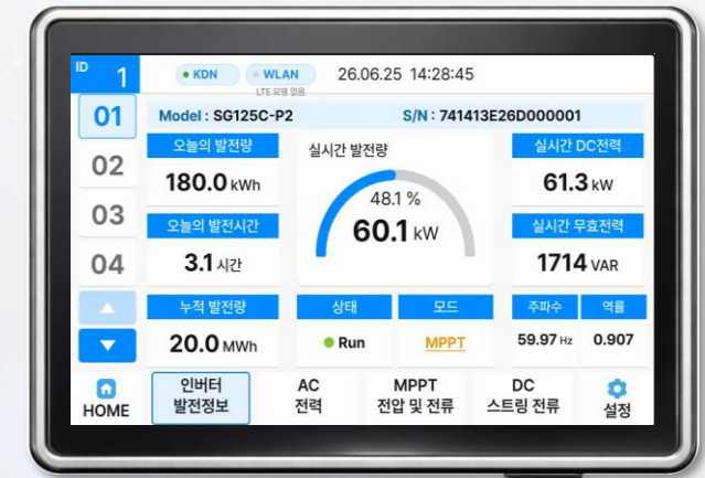
HMI Inverter Monitoring
